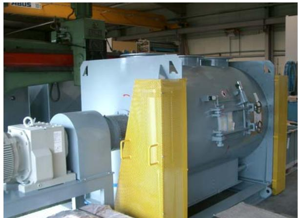
If there are frequent changes in formula or colour, the usage of the AVA batch mixer is recommended, as experience shows that generally more than four components are used and several formula changes are undertaken per day. The degree of automation is variable, as even the smallest quantities of components can be charged into the mixer by means of a manual hopper
